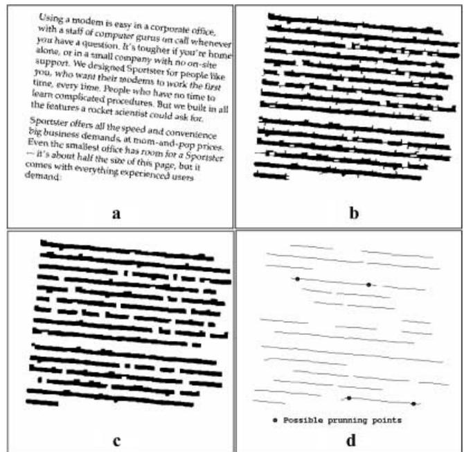
**Fig. 2a.** Original document in binary **b** closing original binary image with  $4 \times 12$  SE **c** opening the closed image with  $5 \times 5$  SE **d** after transition and rejection of small lines operation
