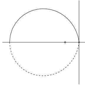
Figure 7.6: Map of the contour  $\Gamma$  under the map  $L(s) = \frac{s+2}{s^2-1}$  given by (7.3). The map of the positive imaginary axis is shown in full lines, the map of the negative imaginary axis and the small semi circle at the origin in dashed lines.
