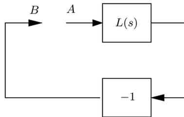
Figure 7.2: Block diagram of a simple feedback system.
