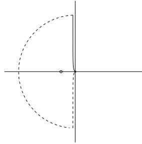
Figure 7.5: Map of the contour  $\Gamma$  under the map  $L(s) = \frac{k}{s(s-1)(s+5)}$ . The curve on the right shows the region around the origin in larger scale. The map of the positive imaginary axis is shown in full lines, the map of the negative imaginary axis and the small semi circle at the origin in dashed lines.
