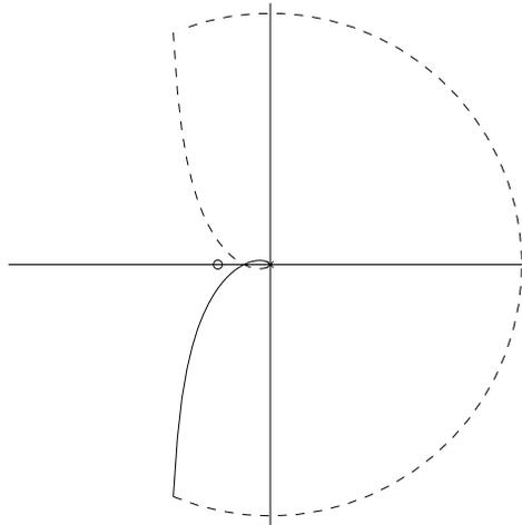
Figure 7.4: Map of the contour  $\Gamma$  under the map  $L(s) = \frac{k}{s((s+1)^2)}$ . The curve is drawn for  $k < 2$ . The map of the positive imaginary axis is shown in full lines, the map of the negative imaginary axis and the small semi circle at the origin in dashed lines.
